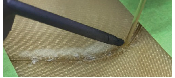
Figure A-5: Filament welding two sections together.
