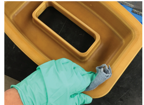
Figure 6-18: UAV bulkhead tool being prepped for use.
