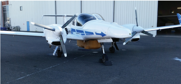
Figure 6-5: Composite belly pod fairing installed on Centaur aircraft (before and after painting).
