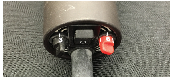
Figure A-3: Fan and temperature settings for ULTEM 1010 resin if using a Leister Hot Jet S hot-air hand tool.
