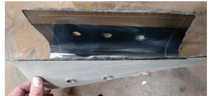
Figure 6-10: FDM tool in ULTEM 1010 resin (top) and resulting part (middle, bottom).
