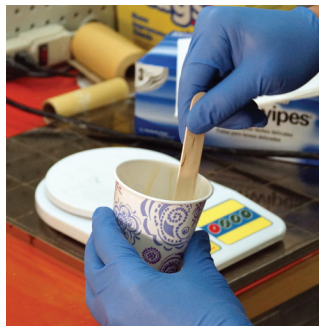
Figure B-3: Mixing the epoxy.
