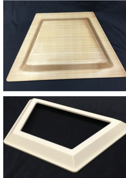
Figure 6-12: FDM tool in ULTEM 1010 resin (top) and corresponding trim tool (bottom) for a blocker door, pan-skin tool concept.
