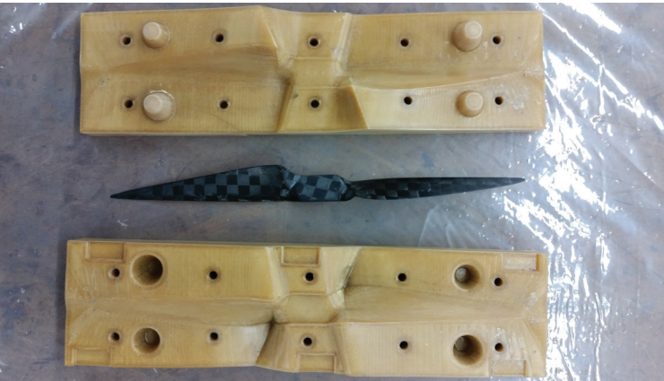
Figure 6-7: Carbon/epoxy composite propeller blade produced on a compression mold tool made from ULTEM 1010 resin
