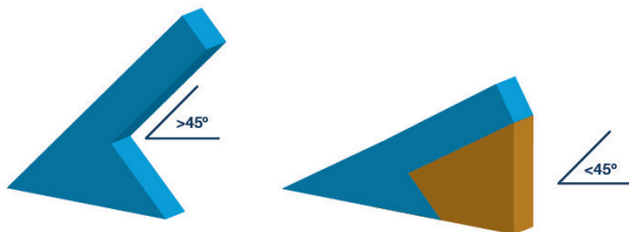
Figure C-5: Self-supporting angles (left) require no support material.
