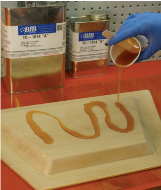
Figure B-4: Pouring epoxy on the tool.
