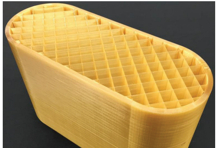
Figure 3-2: Test coupon for structural integrity testing of envelope-bagged, sparse style (sparse double dense in Insight), ULTEM 1010 resin. Raster spacing of 0.5 inch is shown.
