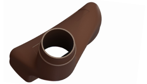
Figure 4-4: An additional shelling step creates a shell tool from a sparse tool.
