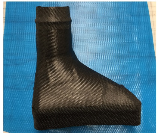
Figure 8-1: Follow standard lay-up procedures when using FDM sacrificial tooling.
