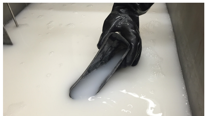
Figure 10-2: FDM sacrificial tooling easily washes out in a detergent solution.
