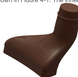
Figure 4-3: Extending open faces and adding trim lines and locating features assist in the lay-up and post-processing of the composite part.
