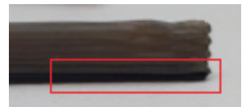
Figure 5-12: Two layers of ST-130_S support material are automatically generated underneath the stabilizer wall, ensuring that it adheres to the build sheet.
