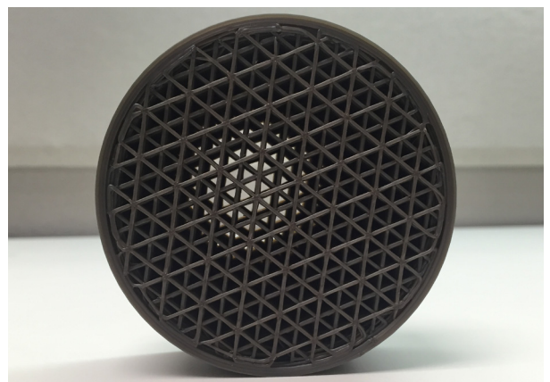
Figure 5-3: The interior fill pattern custom created for FDM sacrificial tooling provides a path for fluid flow.
