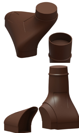
Figure 4-6: Tools that are larger than the build chamber of the machine must be sectioned in CAD.
