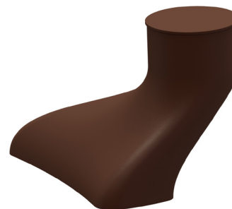
Figure 4-2: A solid body is created by extracting the interior surface of the composite part by closing open areas (top). Hiding the composite part reveals the sacrificial tool (bottom).
