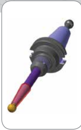
Set clearances for any part of the tool or holder
