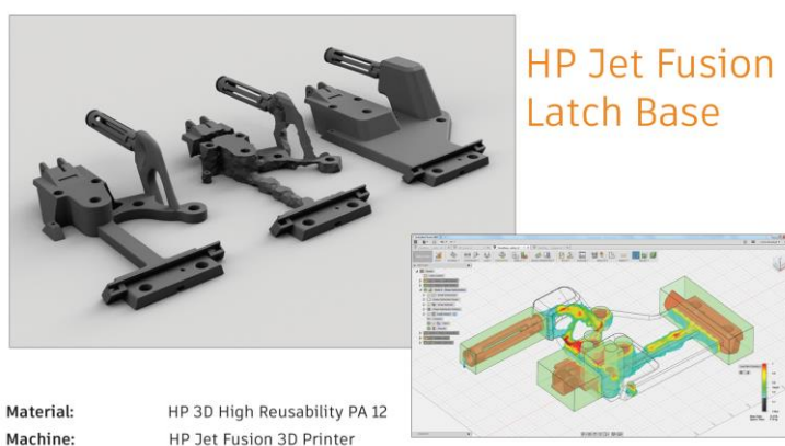
Figure 18: An example of various topology optimization iterations of an industrial part. Deep knowledge of the geometry and performance requirements of the part is required.
