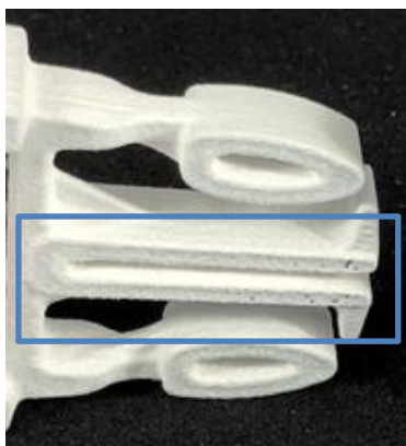
Figure 25: An example of voids caused by bubbles.
