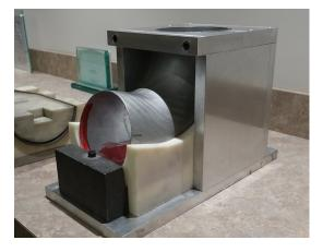
Expansion die used to expand the end of a tube approx. 100 thousandths of an inch. 3D printed ABS insert to hold tube in proper location.
