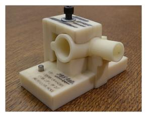
Experimental job - Machining fixture with an actual 3D print of the part, providing a visualization of the part before it was produced. Fixture holds part at the proper angle allowing for simple machining with an end mill. "Doing a fixture like this out of metal would be either next to impossible or very expensive". -Skip Charest
