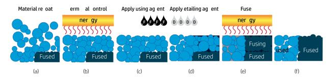
The process begins by recoating the material in a thin layer across the work area, as shown schematically in Figure 2a.
