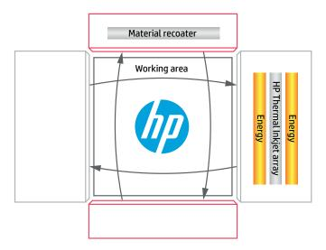
In an HP Jet Fusion 3D Printer, a part, or a set of parts, is built layer-by-layer over a working area inside an HP Jet Fusion 3D Build Unit. After job completion, the build unit is rolled into an HP Jet Fusion Processing Station for cooling, unpacking the parts, and recovery and refreshing the build material. While those processes are completing, a build unit that has been refreshed by the HP Jet Fusion Processing Station can be rolled back into the printer for continuous production. 6
